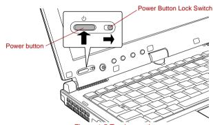
Figure 1-5 Turning on the power
